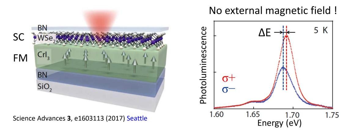
Zeeman splitting  $\Delta E$  equivalent to an effective magnetic field of 13 T ! Circular polarization  $\rightarrow$  could be due to spin dependent charge transfer
